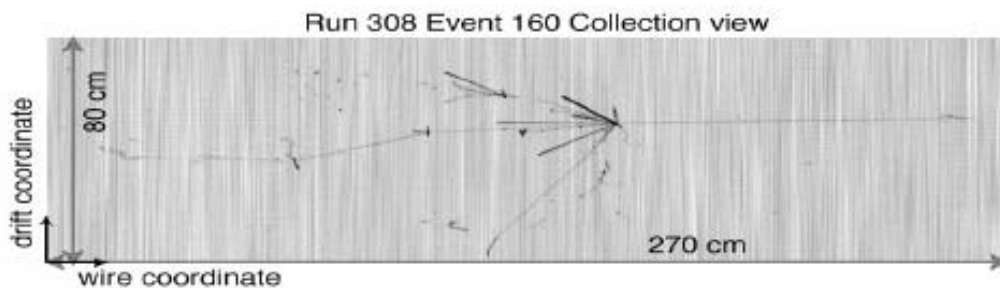
Figure 5. View of an hadronic interaction recorded in the T600 test run in Pavia.
